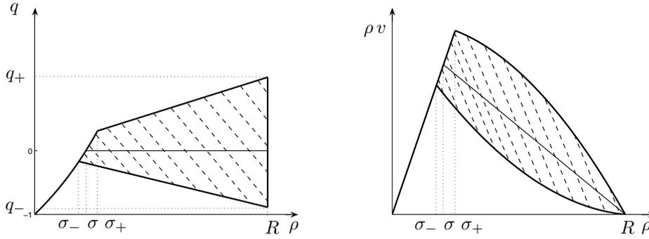
FIG. 3.4. *Newell-Daganzo equilibrium flux function. Left: Fundamental diagram in state space coordinates. Right: Fundamental diagram in flux-density coordinates. The equilibrium is the usual triangular diagram as in figure 3.3. A two-dimensional off-equilibrium set of parameters (striped domain) is modeled in congestion.*
